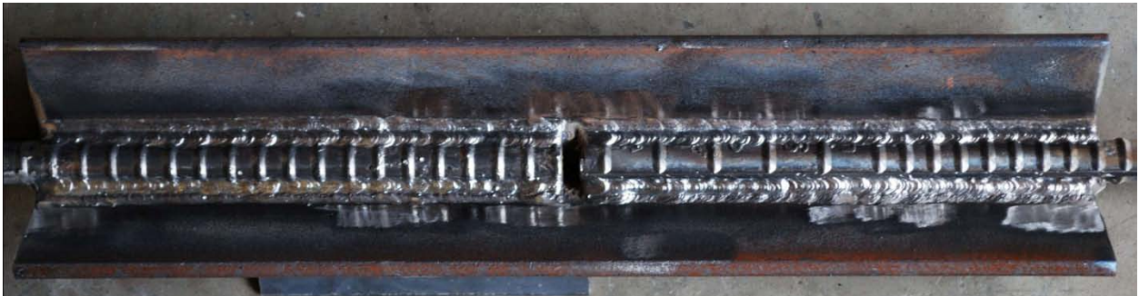
Completed weld (3 passes).
